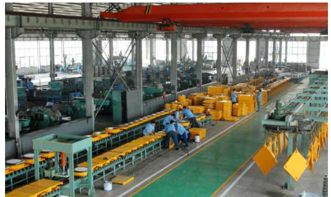
The assembly of pot bearing in the workshop.
