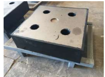
Rectangular lead rubber bearing with four lead core.
