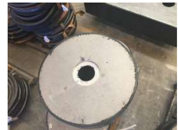
Round lead rubber bearing with single lead core.
