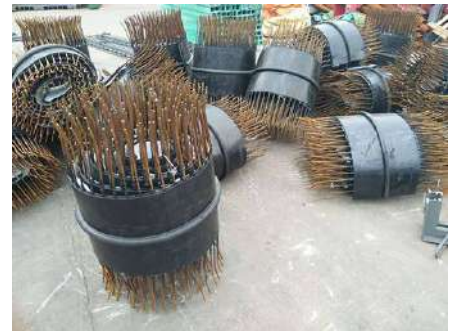
Implantable expansion joint rolls has simple structure
